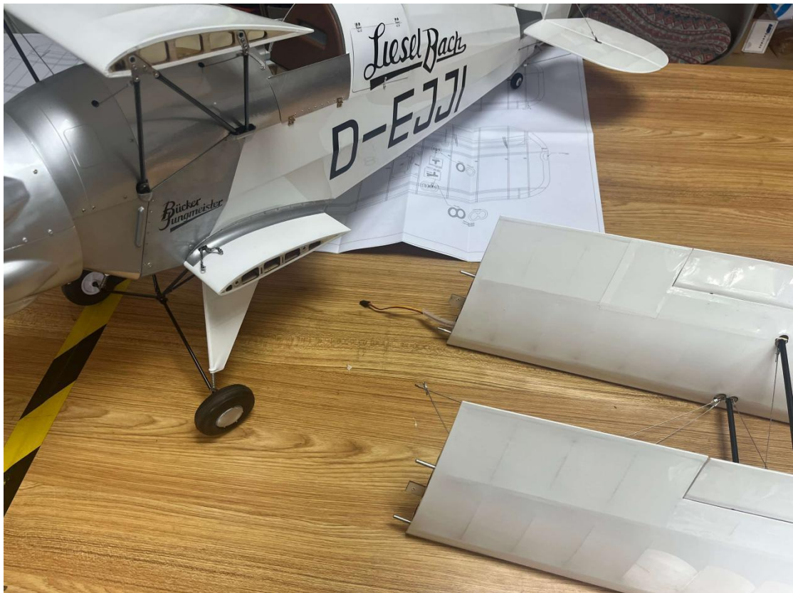
How to remove the wings: Step 3 – Remove bottom wing
