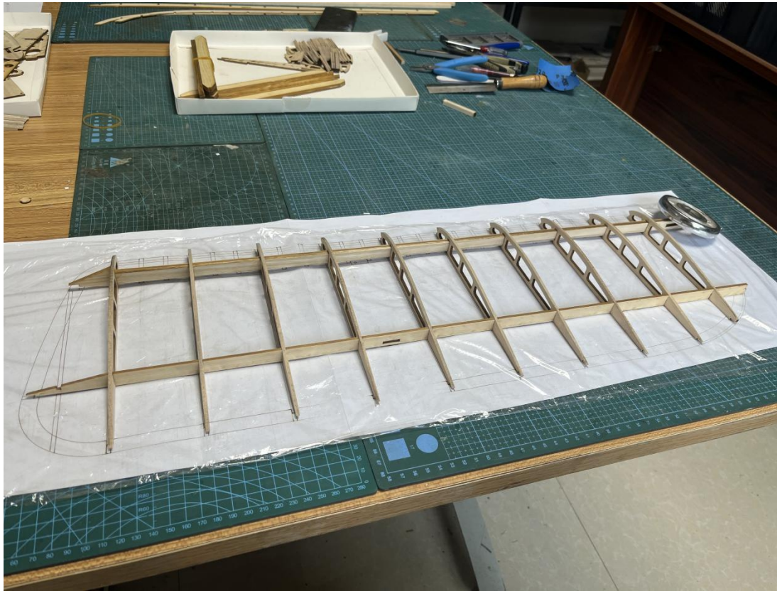
Step 18: 6 x 6 mm Balsa Strips.
